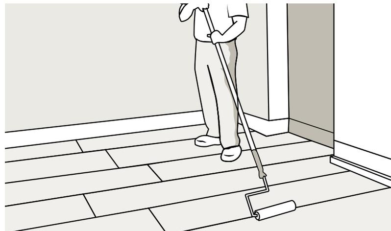
Figure 3: The main application of the lacquer should be with a long-handled roller.
